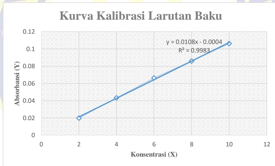
Gambar V.8 Kurva Kalibrasi Larutan Standar Timbal
